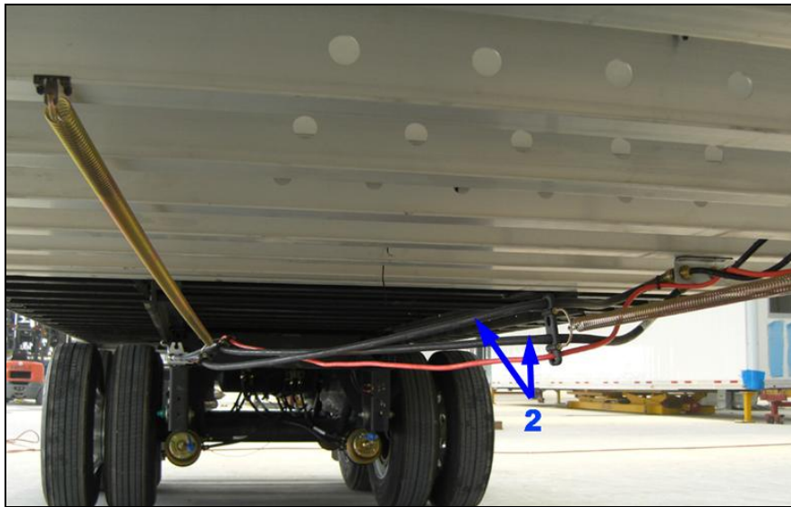
Figure 7-4 - Check Air Hoses
