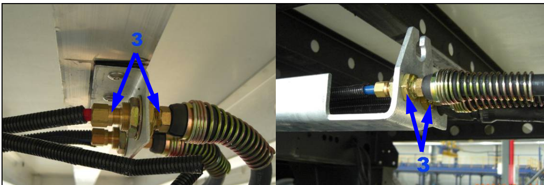
Figure 7-5 - Inspect Air Fittings
