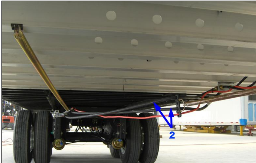
Figure 3-8 - Check Air Hoses
