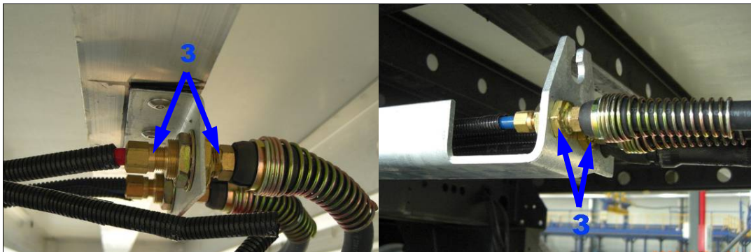
Figure 3-9 - Inspect Air Fittings
